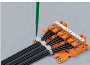
Horizontal mounting with strain relief plate on flat surface. Wiring locations identified using marker strips
