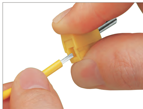
Connection of conductors via banana plugs: Press button fully and insert stripped conductor into square entry and release
