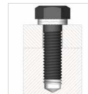
Hexagon bolt secured in a blind hole
