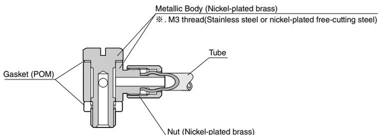
※ . Gasket material for metric thread: SUS304+NBR or POM for standard specification : POM for Clean-room package
