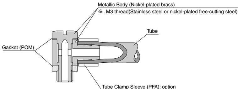
※ . Gasket material for metric thread: SUS304+NBR or POM for standard specification : POM for Clean-room package
