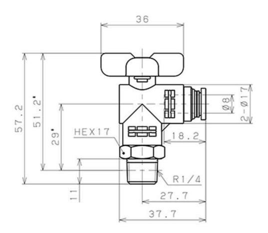
\*The dimension is the one after installation and just for reference.
