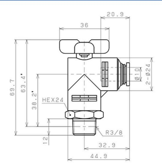
\*The dimension is the one after installation and just for reference.
