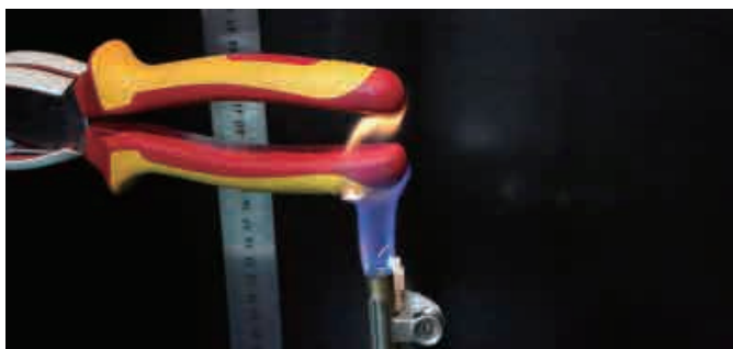
Handle passed flame-retardant test
