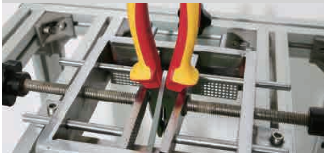
Handle passed 500N drawing force test
