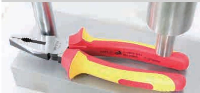
Handle passed impact resistance test
