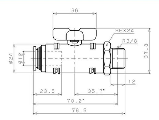
\*The dimension is the one after installation and just for reference.
